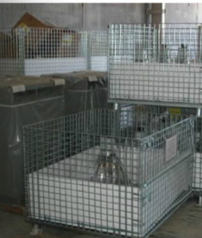
FIGURE 7: Pre-assembled high-bay fixtures shipped in collapsible bins, courtesy of Cleveland Electric, 2003.
