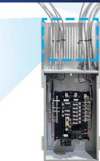
Prepare Load Centers in the shop, ready-to install on site!*
