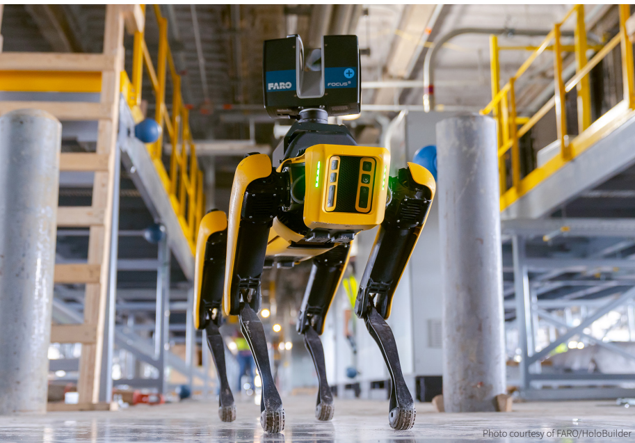
Photo 2. SpotWalk, developed by HoloBuilder, features a 360-degree camera on the robot's back, eliminating the man hours and potential injury of sending employees to do that documentation manually.
