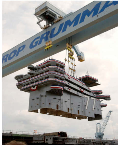
Figure 37: The Final Superlift on the George H. W. Bush Island
